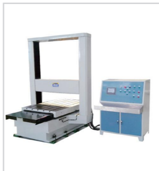
HBM-3000C 大型门式电子布氏硬度计 Large-Sized Gantry-Mode Electric Brinell Hardness Tester
